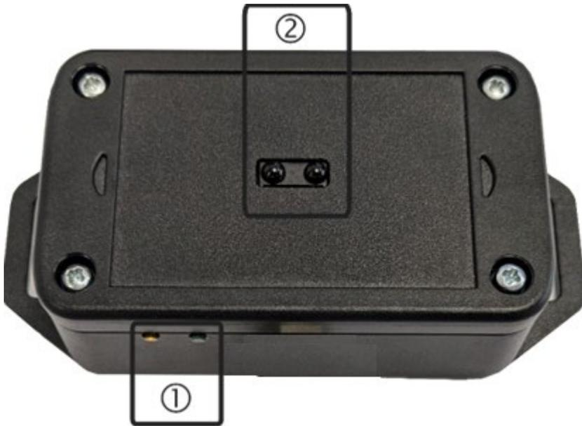
**Fig. 2: Optical transceiver unit with supply cable**
