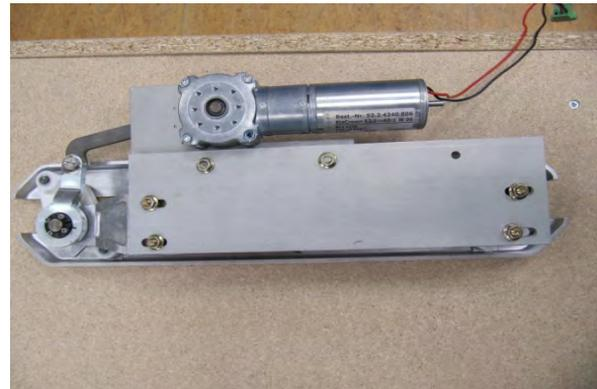
**Abb. 18: Motor mounted on the drive TL**
