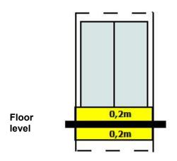
Fig. 5: Schematic representation of the unlocking zone
