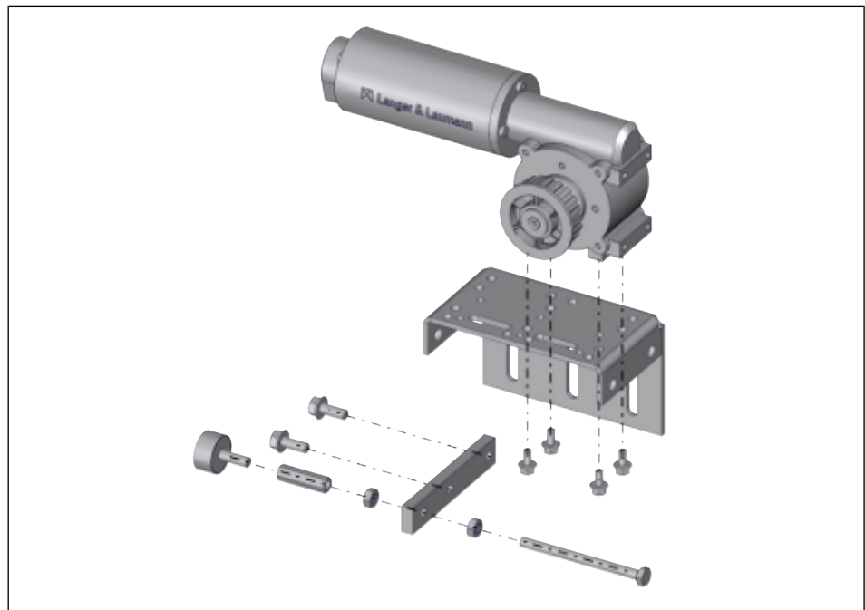
III. 14: Assembly of the drive unit
