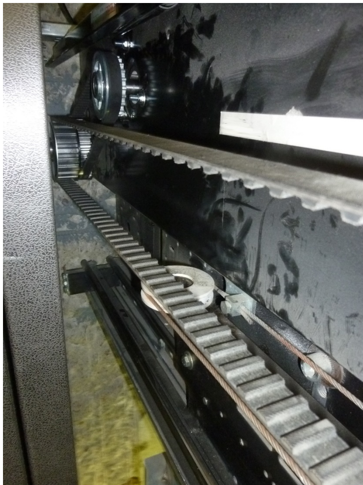
Fig. 18: Door machine with TSG, completely mounted (centre opening)
