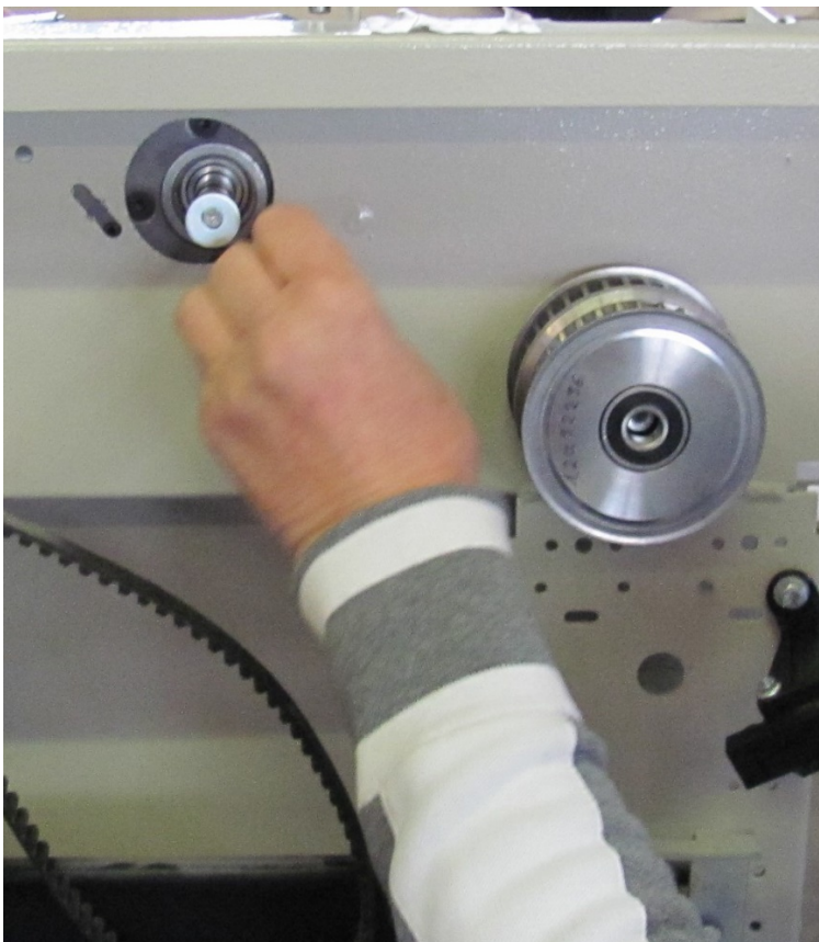
Fig. 13: New double belt sprocket, mounted and TSG drive (still without pinion)
