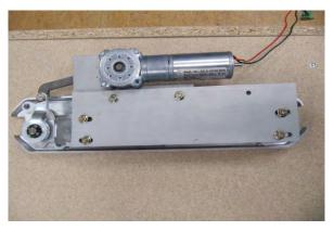
Abb. 18: Motor mounted on the drive TL
