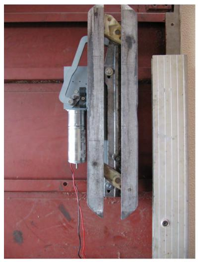
Abb. 14: View mounted drive motor at TL
