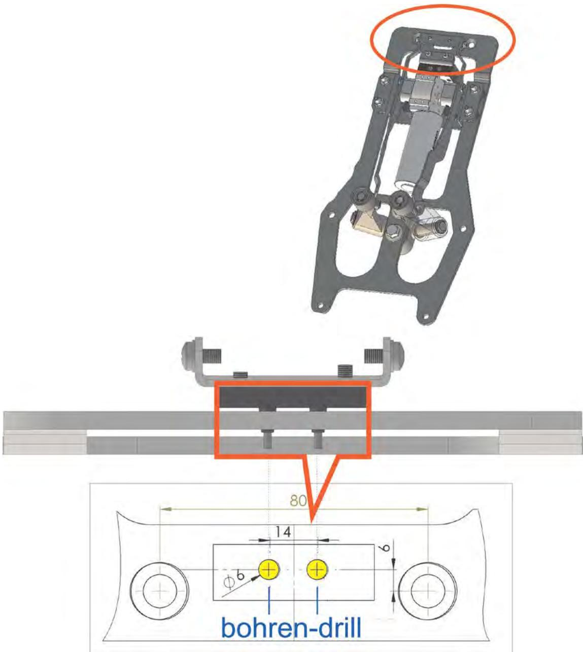
Abb. 10: Processing door (drilling pattern)
