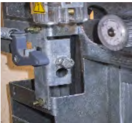
Fig. 3: Stop provided by an 8 mm screw
