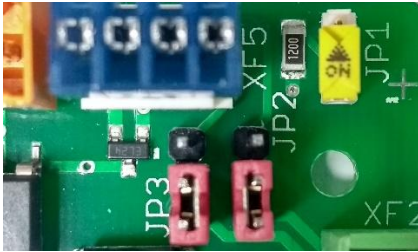
Fig. 7: Default setting, 24V supply via XF2
