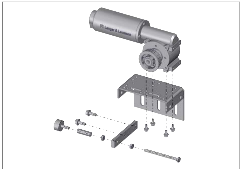
III. 14: Assembly of the drive unit
