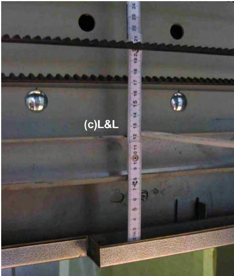
Abbildung 6: Height of track of car roof (car internal height)
